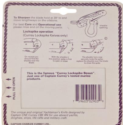
To Sharpen the blade hold at 20° to and move lengthways on the oilstone.
